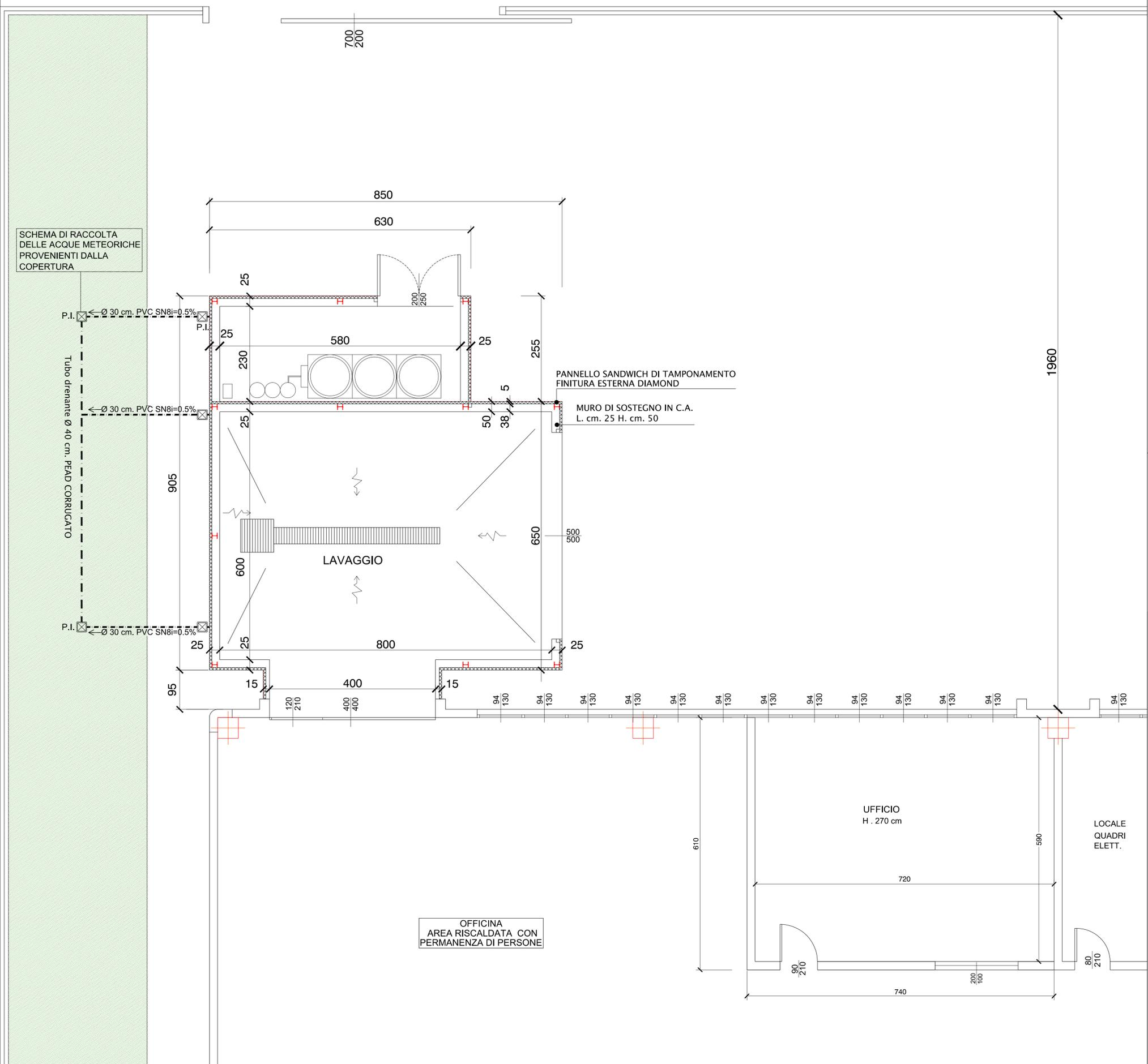
SCHEMA DI RACCOLTA DELLE ACQUE METEORICHE PROVENIENTI DALLA COPERTURA
